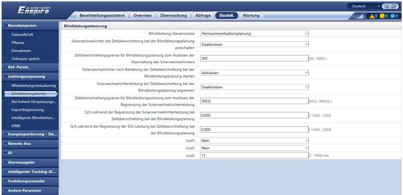
The screenshot shows the 'Einstell.' (Settings) tab in the Enspire software. The 'Blindleistungssteuerung' (Blind Power Control) section is active. The 'Blindleistung-Steuermodus' (Blind Power Control Mode) is set to 'Fernkommunikationsplanung' (Remote Communication Planning). Other settings include time limits for switching solar inverters and compensation limits for solar and ESS, with values like 300s, 300.0s, and 0.000.
