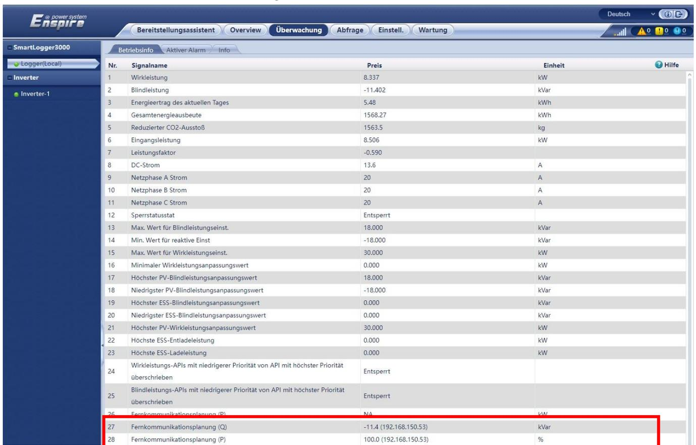
The screenshot shows the 'Überwachung' (Monitoring) tab in the Enspire software. A table of signals is displayed, with the last three rows highlighted in red:
